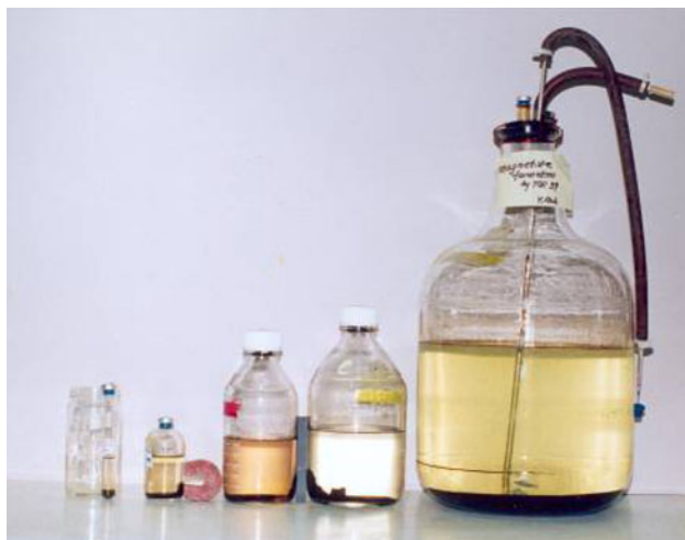
Fig. 1 Prototype scale-up experiments from 10 ml, 100 ml, 500 ml, 1 l and 12 l of medium
